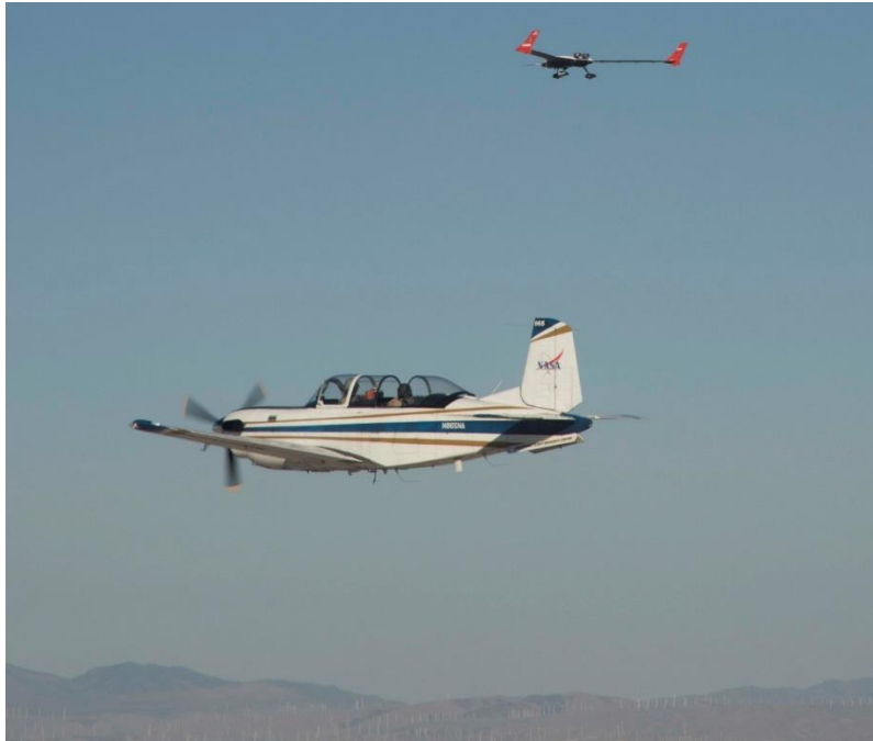
Figure 3.4-1: The NASA T-34C Turbo Mentor (Beech Aircraft Company, now Raytheon Technologies, Waltham, Massachusetts, U.S.A.), a typical chase airplane for the X-56A aircraft.
